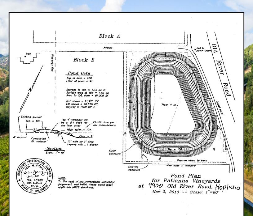
Installed in 2011 13.5 +/- acre feet of water Holds appoximately 4,398,994 gallons of water
